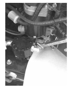
5. If the transaxles are noisy or jerky, purge the transaxles, following the purging procedures. **See Purging Transaxles Page 9**.
