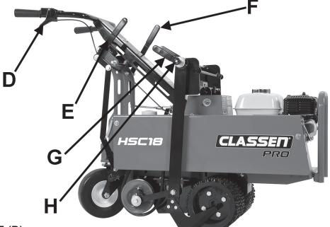
**THROTTLE (D)** - Squeeze the throttle control to increase the engine rpm. Squeezing the throttle control to increase the engine rpm also engages the centrifugal clutch powering the blades and wheels when the blades and/or wheel drives are engaged.
